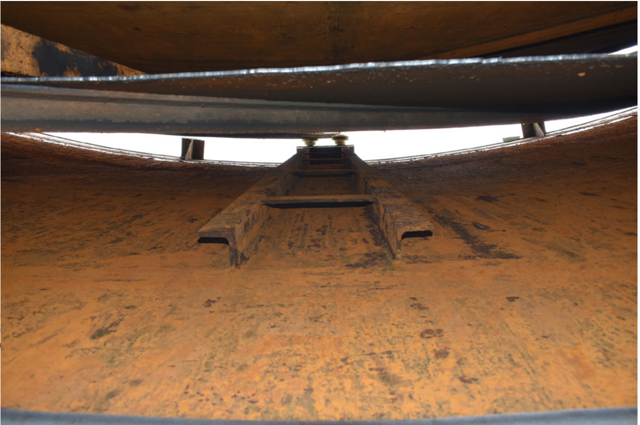
Plate 21: An example of a roller carriage bracket
