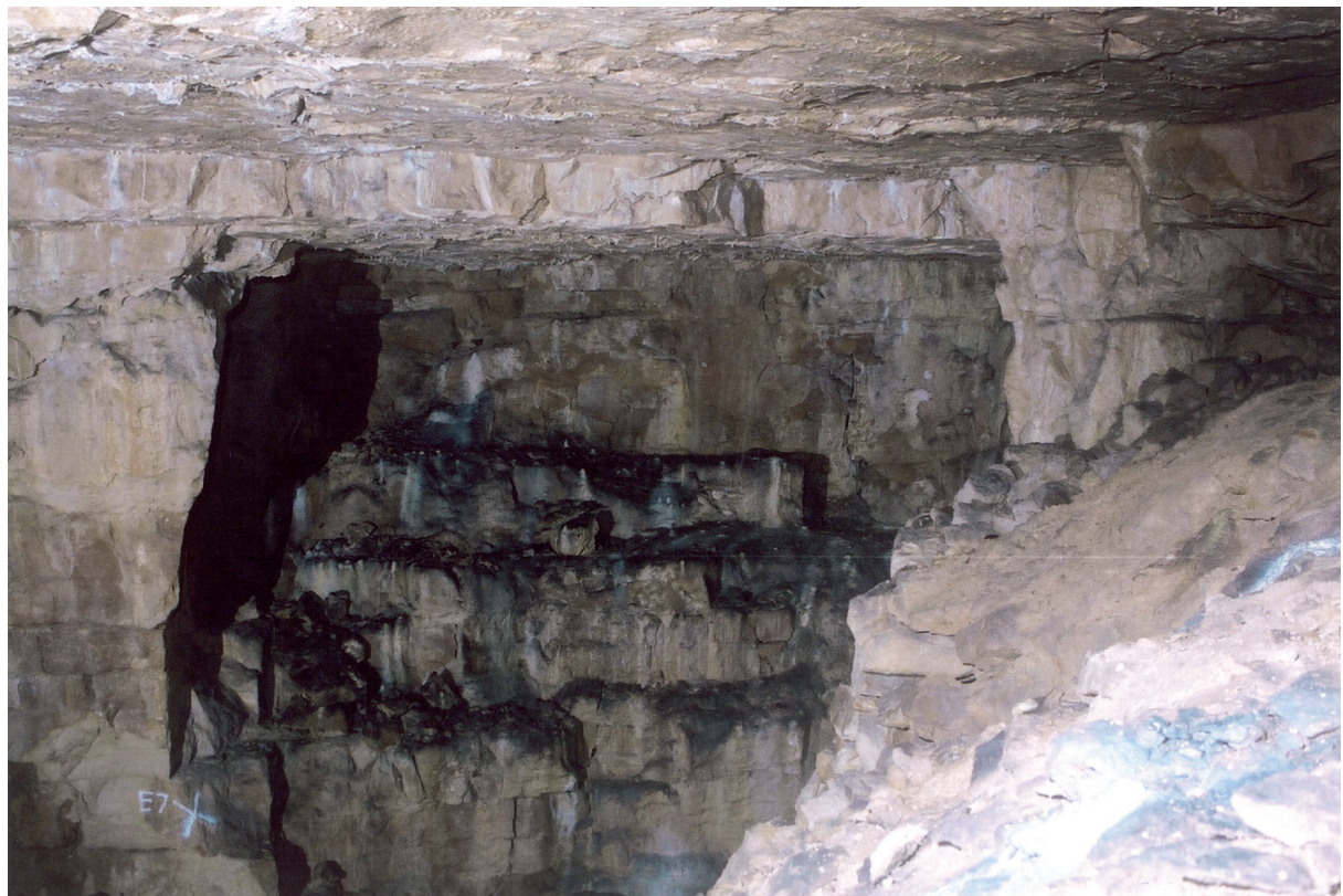
Fig. 7.8 Stepped working face, south-west Firs. This was the only full example found, as usually faces were left vertical or the area backfilled with spoil
