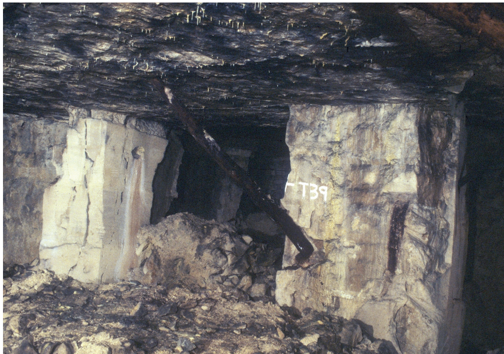
Fig. 8.22 A saw-cut pillar, mid-late 19th century, north Central Firs
