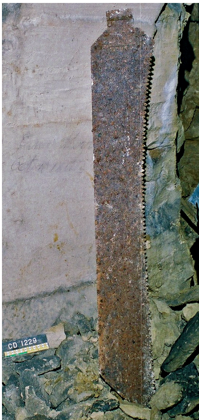
Fig. 8.31 A frig bob saw (late 19th century) leaning against a typical sawn face with graffiti
