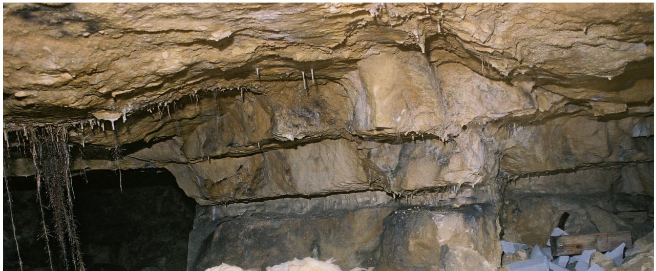
Fig. 8.17 Continuous jad slot across a face
