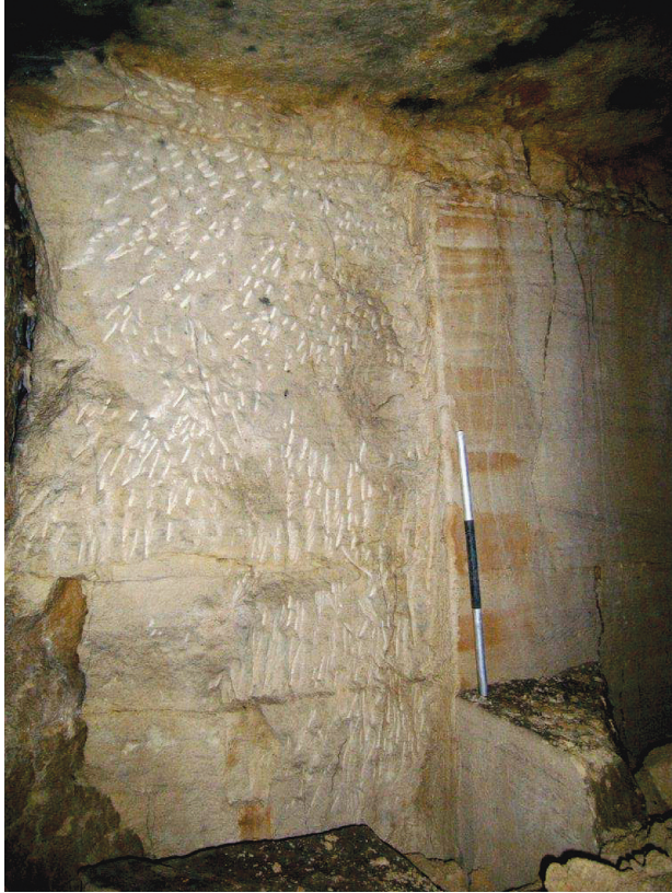
Fig. 8.33 Face in Foxhill Quarry showing picking-back behind the wrist stone to allow insertion of saw behind the sawn face on the right
