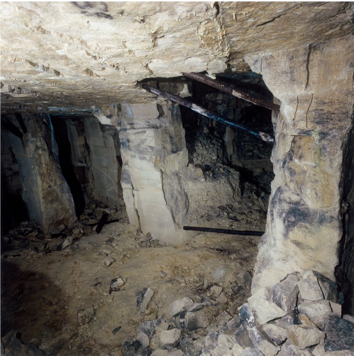
Fig. 8.13 Open Room working area in Byfield Quarry (518). Cranes and winches were used to drag stone away from the working face across the floor. (Photo by Paul Deakin)
