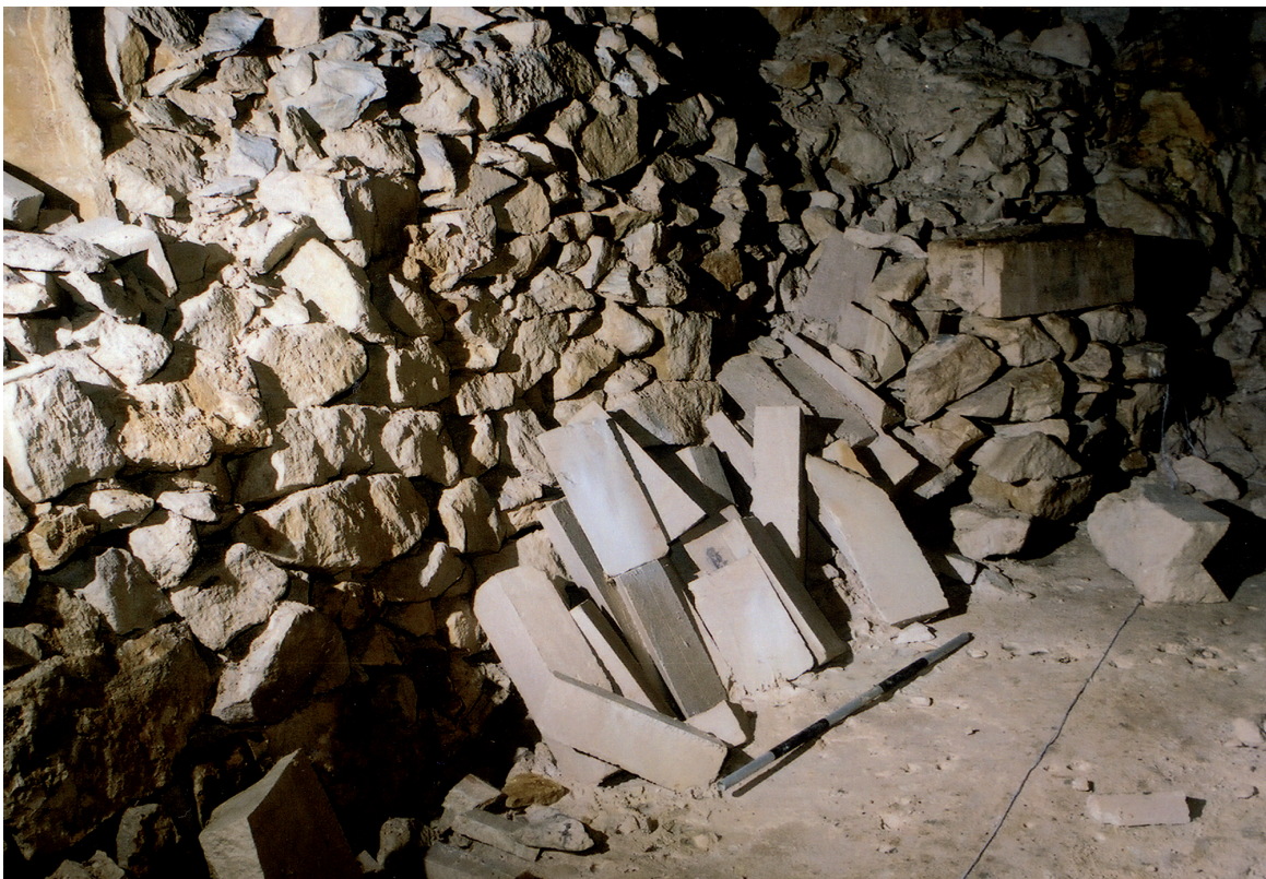
Fig. 8.24 Stacked wrought stone, produced by a banker mason, East Firs
