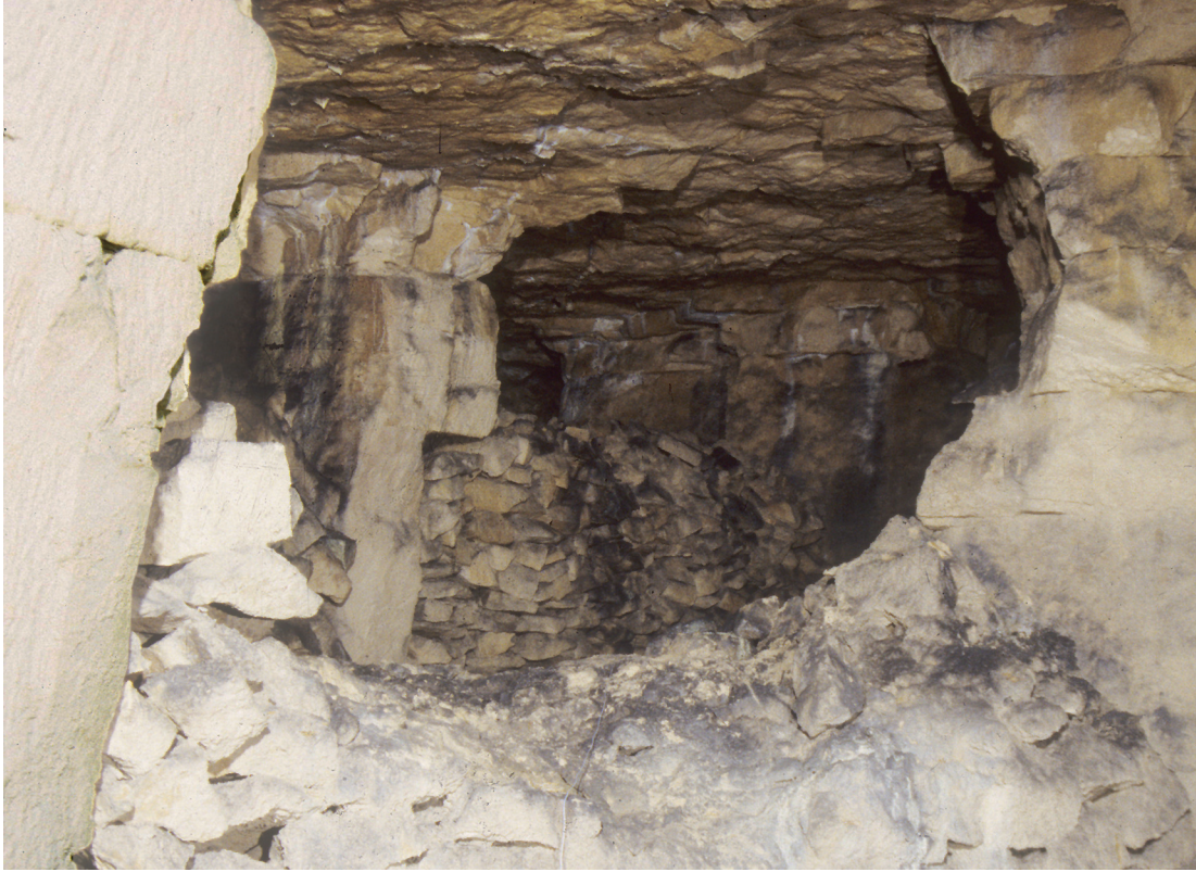
Fig. 8.35 Reworked example of removal of lower block of the best stone. Many examples of this appear to have been deliberately concealed in both East and Central Firs (2201)
