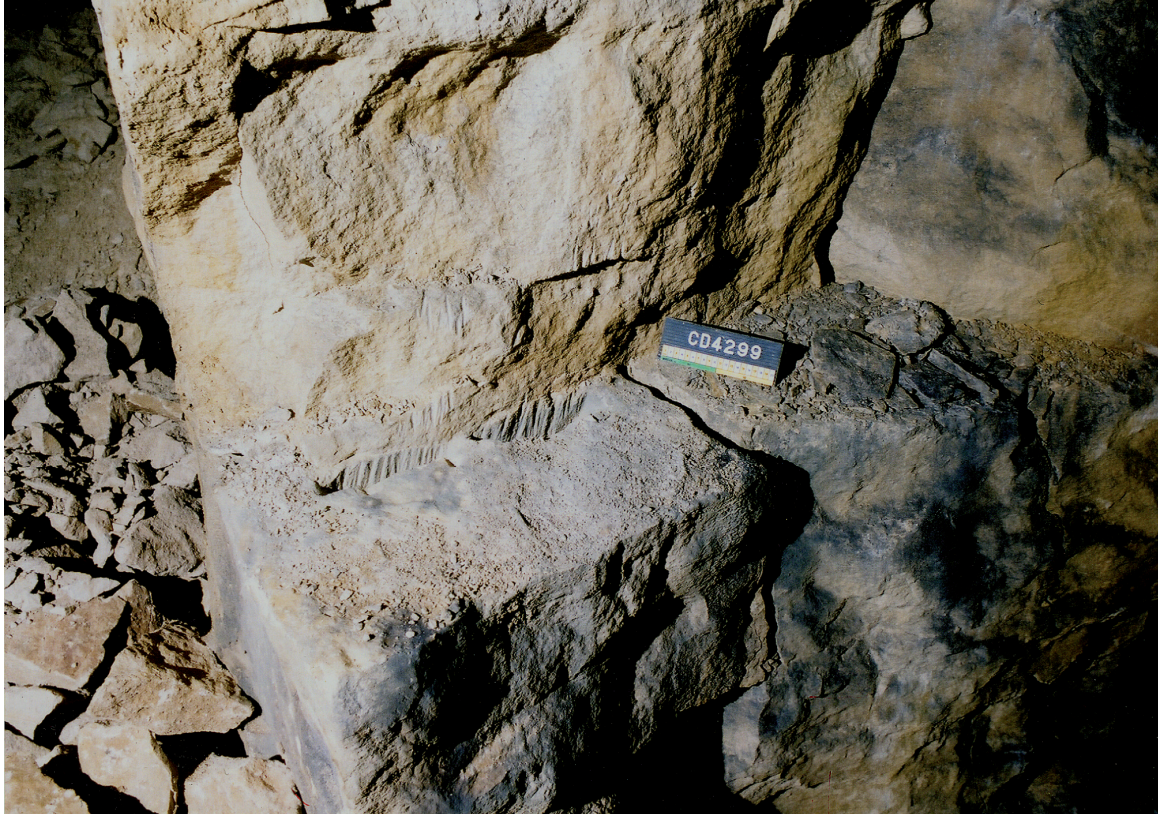
Fig. 8.19 Wedge pits left in situ, East Firs
