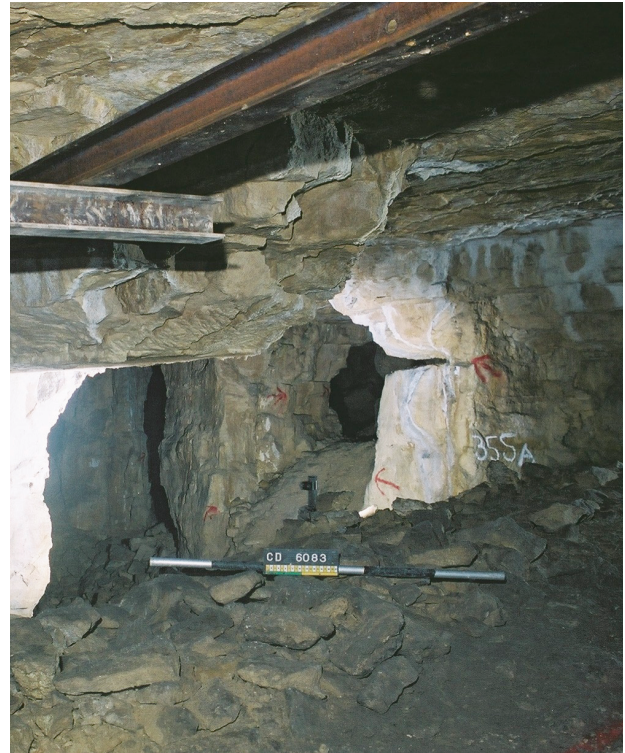
Fig. 8.2 Jad slot near the top of a pillar to allow the bed above or below to be wedged out
