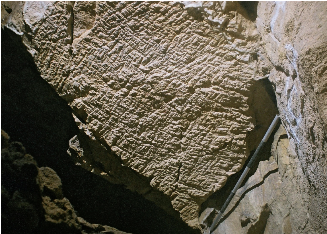
Fig. 8.18 Underside of a jad slot showing pick marks at the rear and jadding iron marks
