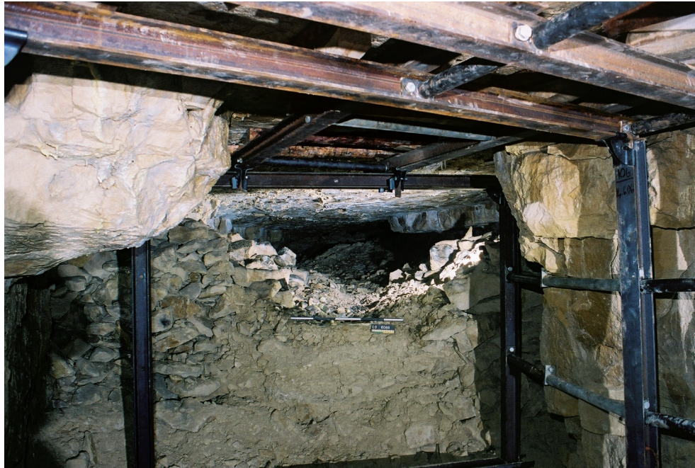
Fig. 9.21 Barrow-way filled in on retreat in Central Firs. The rubble pack rests on the former barrow-way (Quarry Area 2347)
