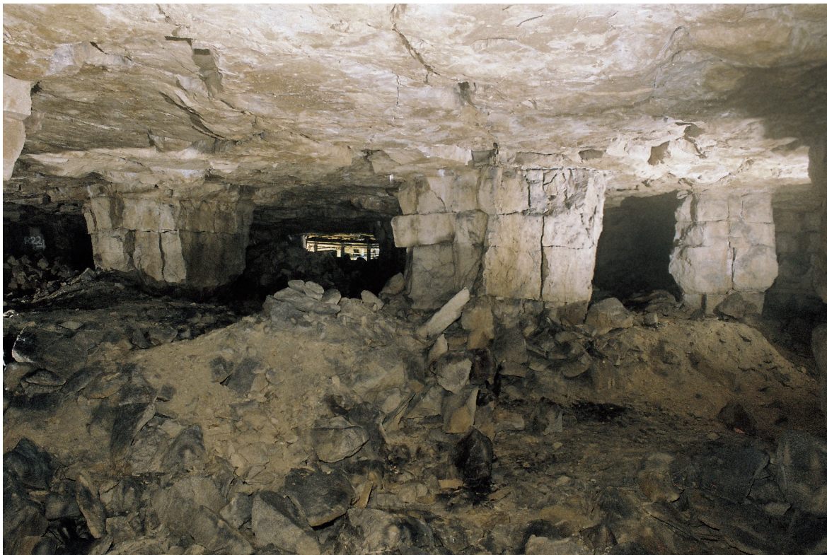
Fig. 10.9 Direct pillars in Central Firs (Quarry 2340)
