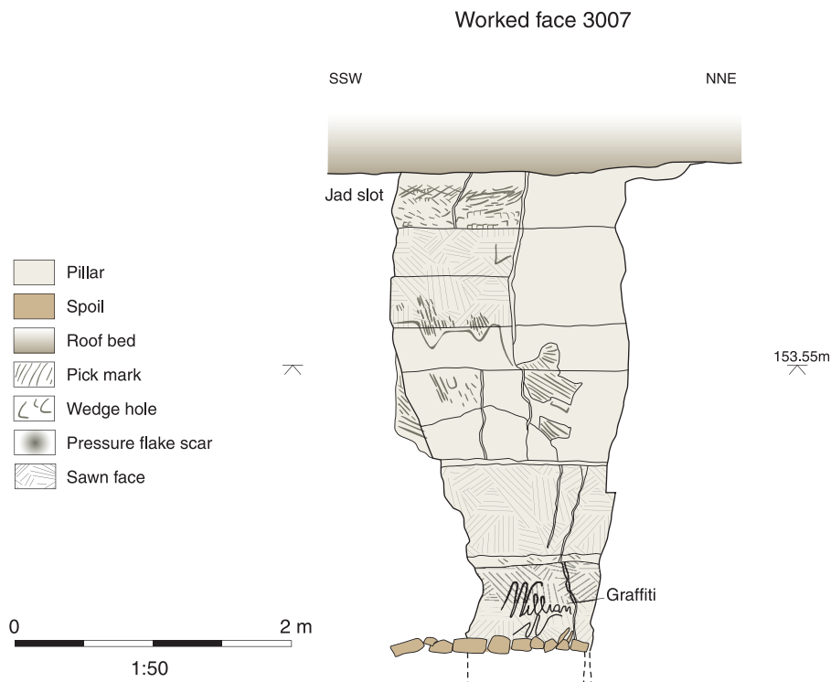
Fig. 10.10 Section of worked face 3007, an irregular form of direct pillar with narrow core, showing picked and wedge and chip broken surfaces
