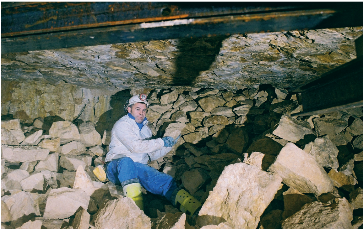
Fig. 10.32 Miner seated in original position demonstrating waste-stowing to roof level
