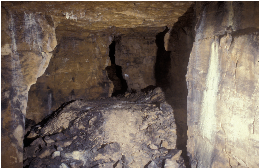
Fig. 10.34 Lobate tipping in Central Firs south of the Grand Canyon (Quarry Area 2209)
