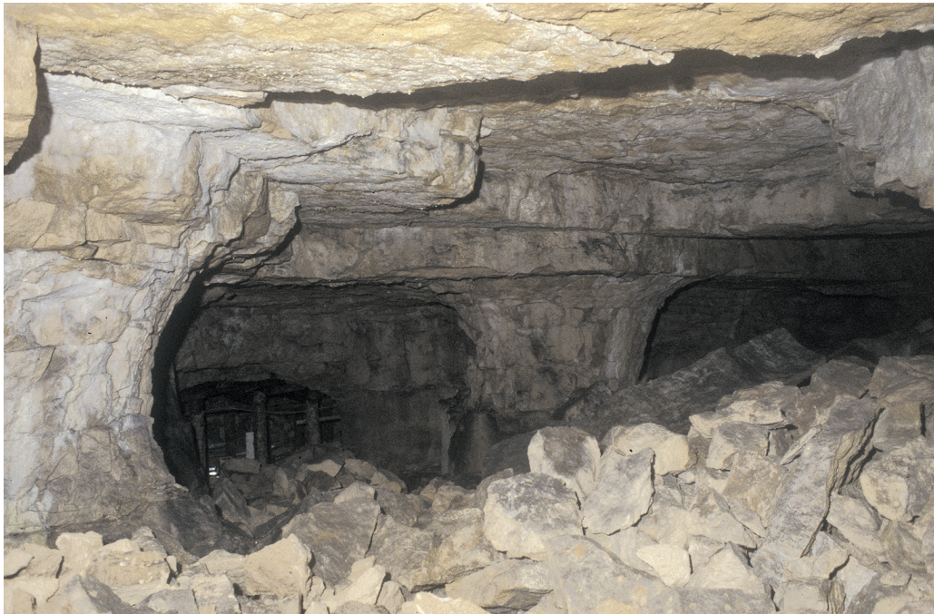
Fig. 10.3 Apophygate pillar in East Firs close to The Brow cartway in Quarry 2339. This is an example outside Allen's quarrying area
