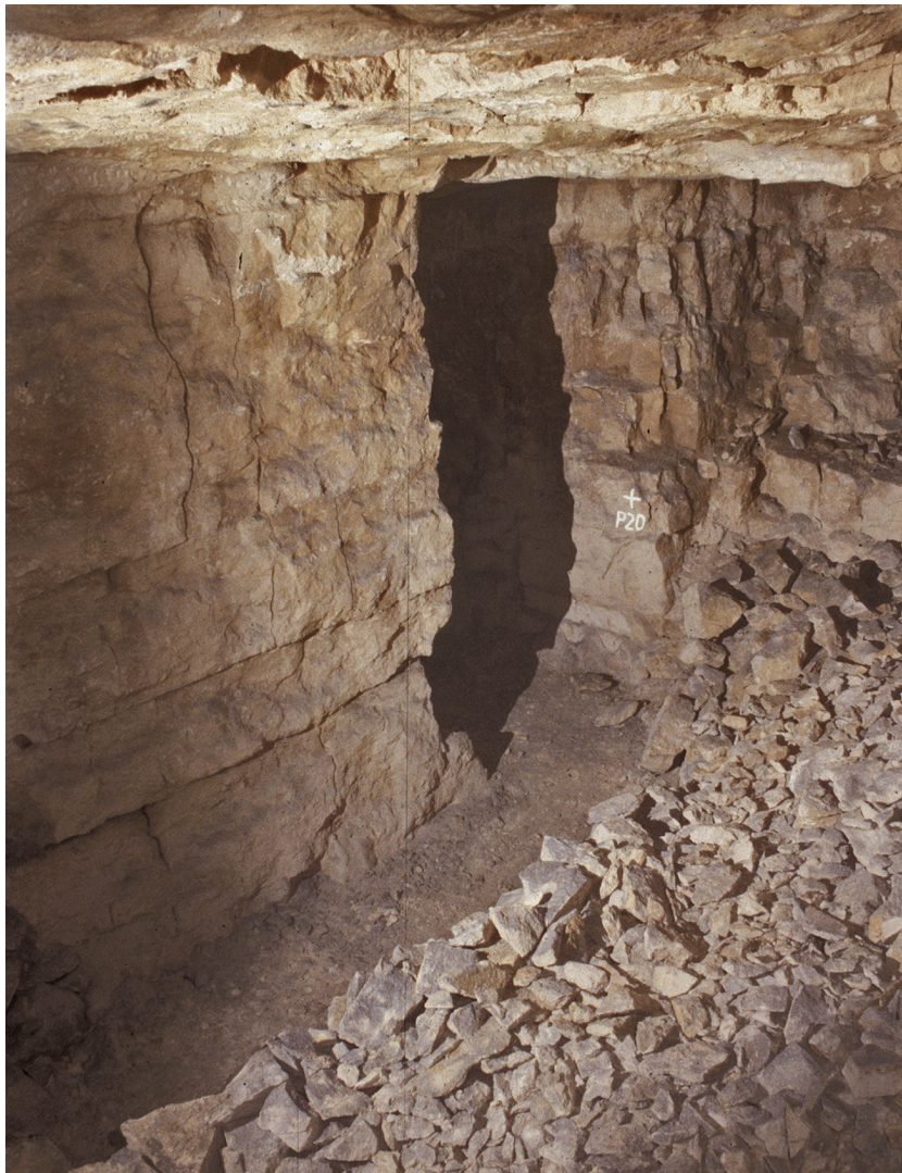
Fig. 12.25 The masons' quarry: note the clear floor, spoil neatly stacked and the clear-cut faces on the pillar
