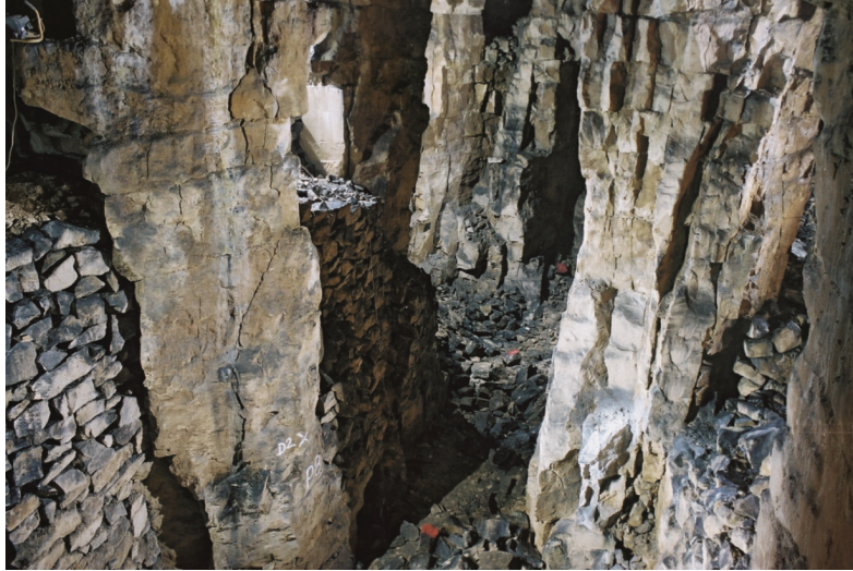
Fig. 12.28 View towards the north-west from just under the roof of the Grand Canyon, directly over the central gullet, showing the full 8.5 m maximum height of the direct pillars and the barrow-way below, with over 5 m-high rubble stone packs at the side
