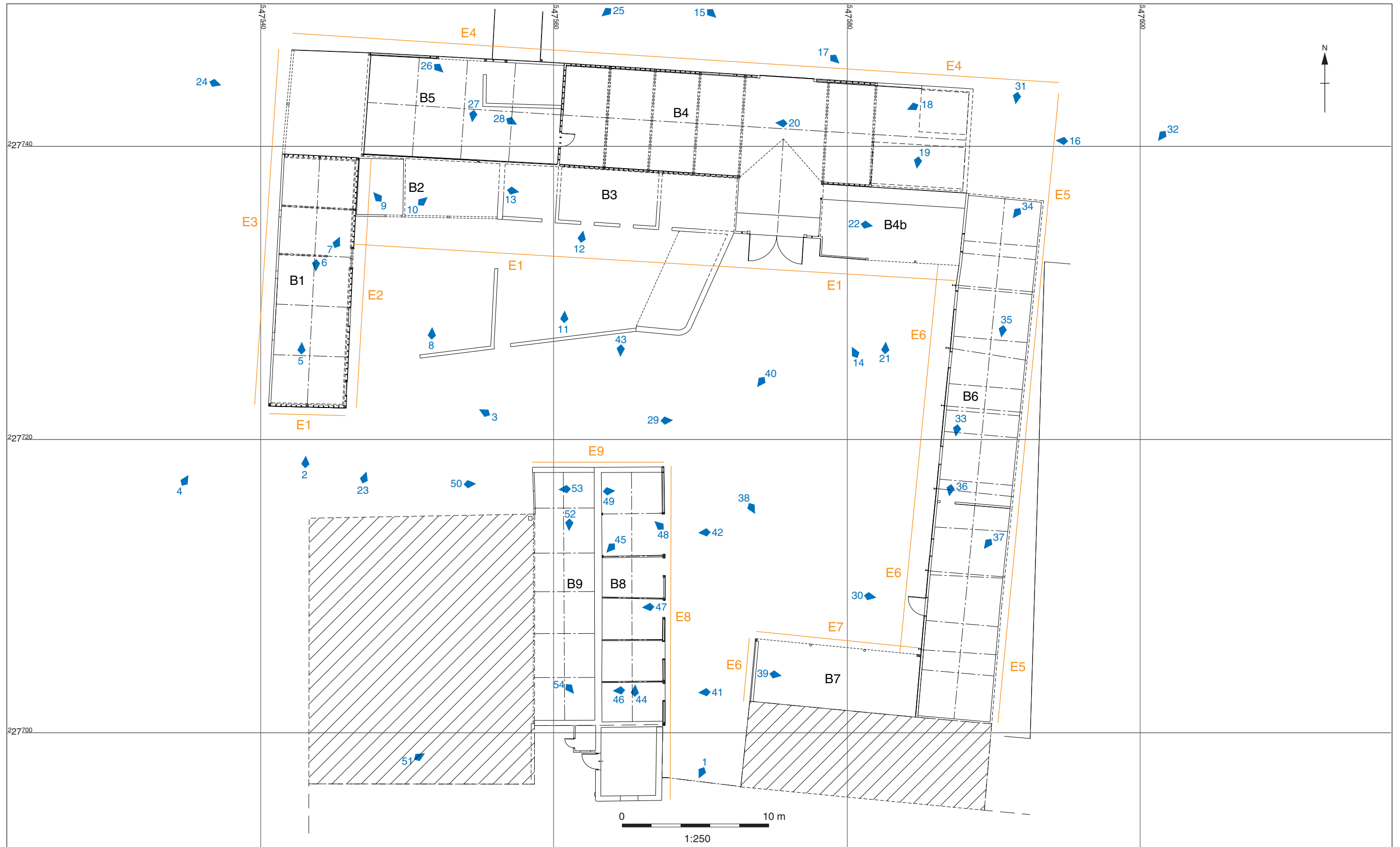
Figure 2: Plan of buildings surveyed showing location of plates and elevations used in report (from data supplied by client)
