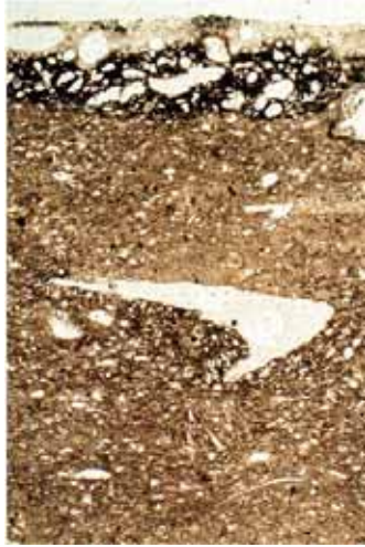
Fig. 13: Photomicrograph of M4240A1 (large 'Green Glaze', Context 4226); plant temper pseudomorphs and 250µm-thick green glaze surface (part of detailed elemental map; see Figs 17-20). PPL, frame height is ~4.62mm.
