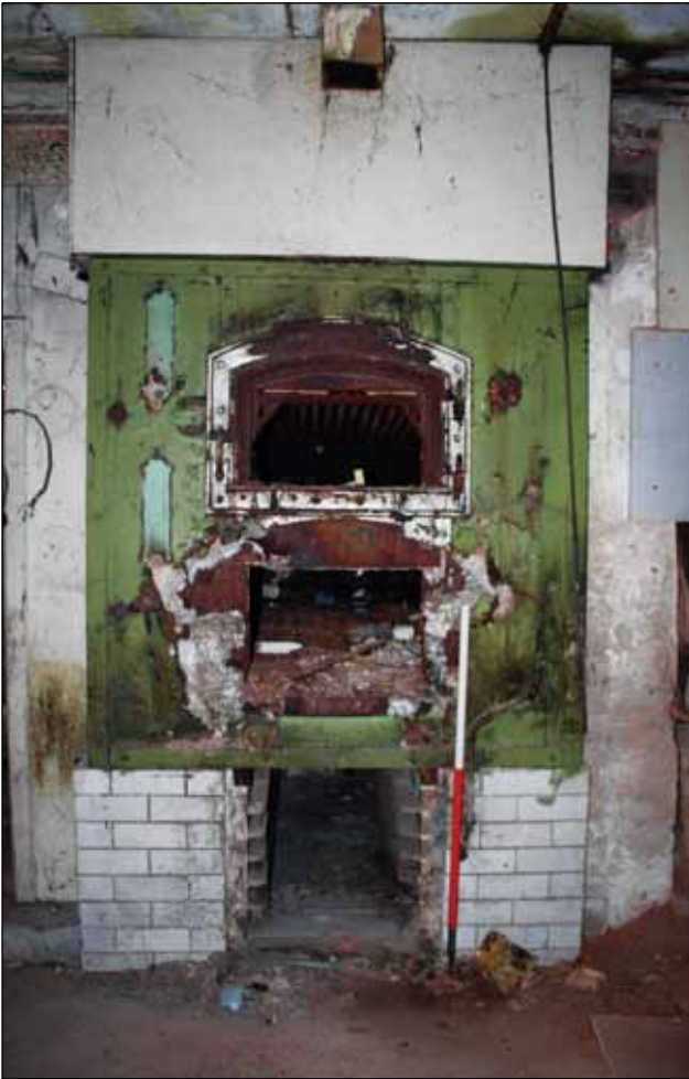
Plate 23: Detail of "Collins Steam Oven"
