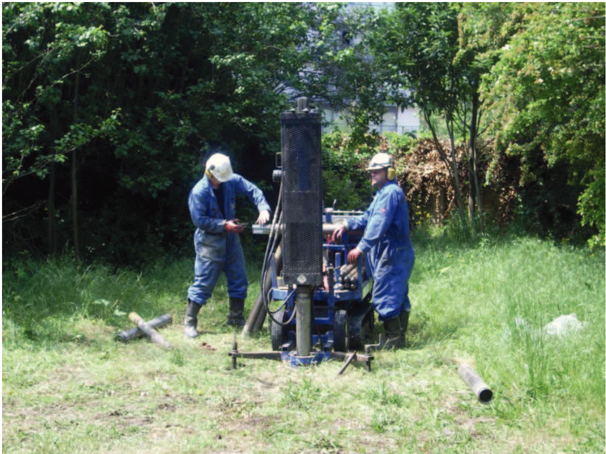
Plate 1: Photo of the borehole sampling - terrier percussion rig
