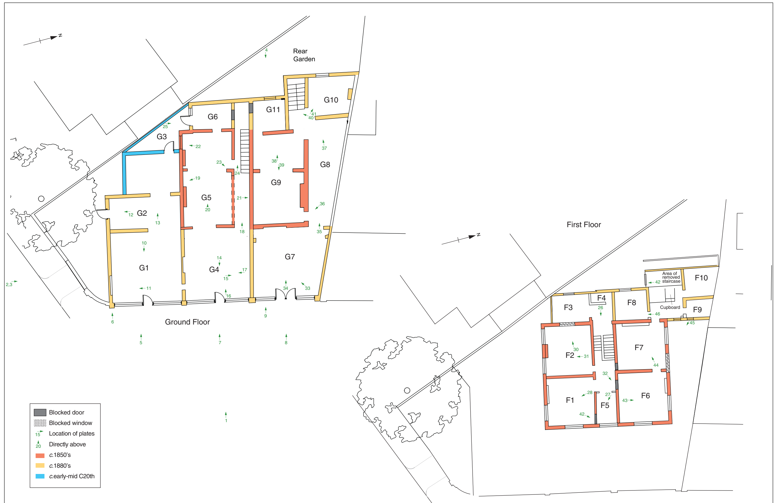
Figure 17. Plan of ground and first floors showing suggested phasing and location of plates referred to in report
