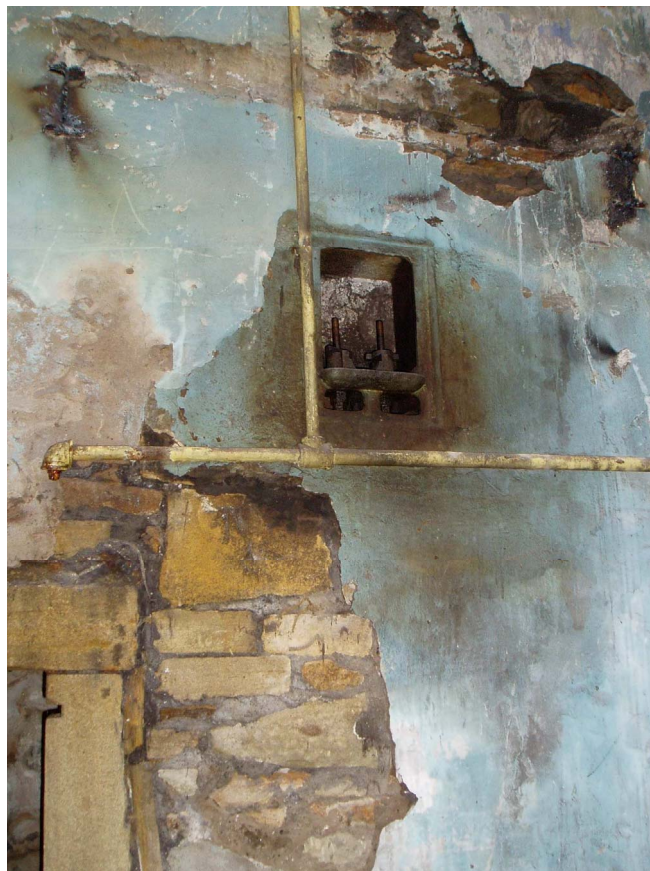
Plate 24: End-carrier bearing for lineshaft, second floor, Building 6
