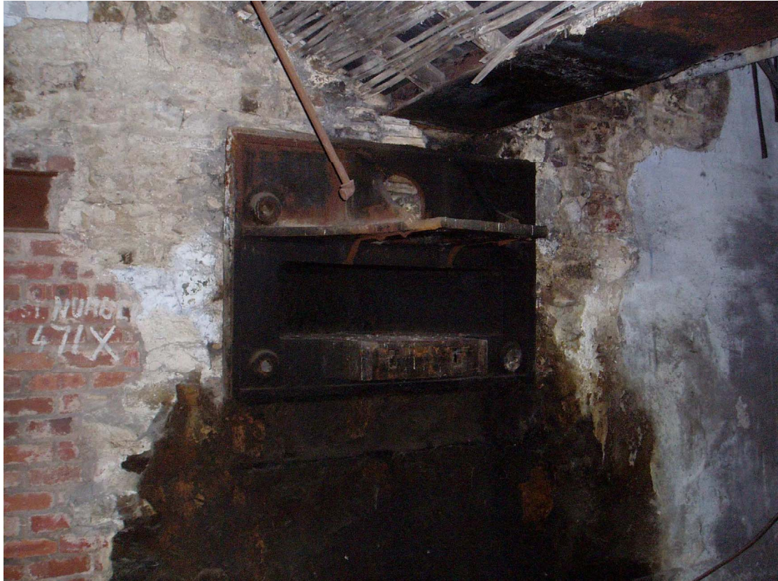
Plate 9: Top steady bearing for vertical driveshaft, Building 1
