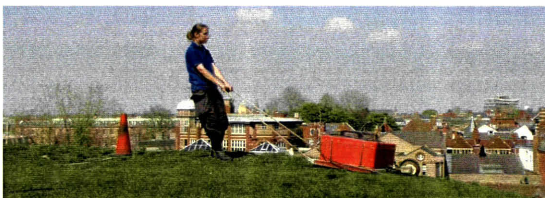
Plate 1: Showing the GPR survey with the 200MHz antenna
