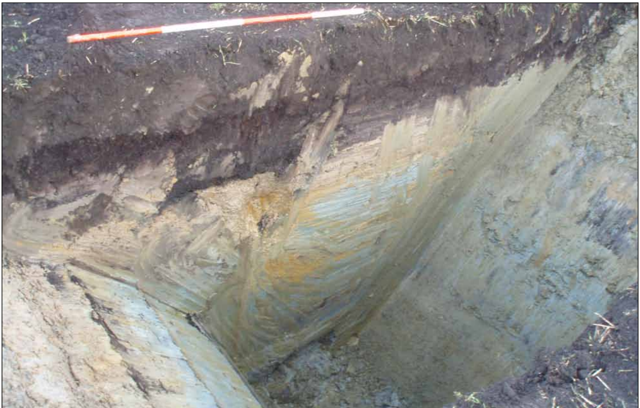
Plate 10: Test pit 8 showing solifluction deposits overlying river gravel
