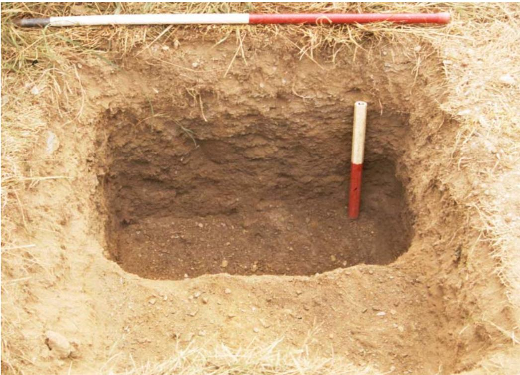
Plate 6: Gravel in base of Test Pit 27
