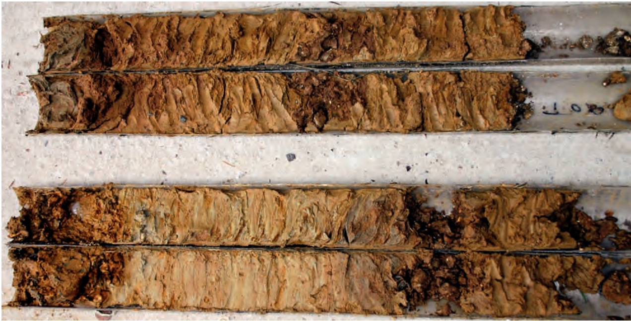
Fig. 2.5 Core samples from West Wittering. Cores are split to show stratigraphy. Fine grained sediments are estuarine deposits sandwiched between two cold stage gravels
