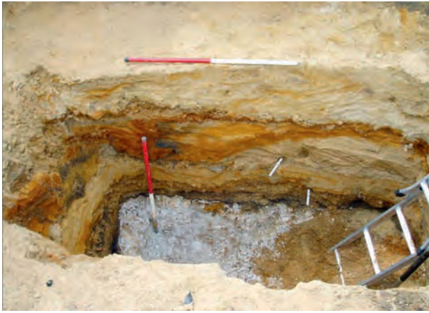
Fig. 2.20 Test pit excavated at Cuxton (Wenban-Smith et al. 2007a) showing fluvial gravels over Chalk bedrock
