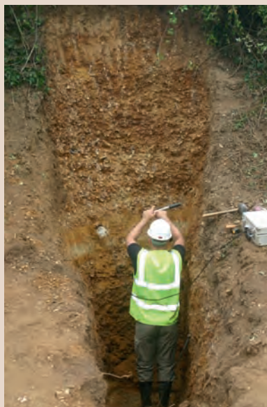
2.5.1 OSL sampling and measurement of radiation from the surrounding environment from a raised beach at St Clement, Jersey
