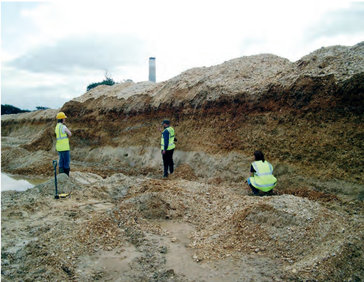
Fig. 2.6 Section cleaning of a gravel quarry face at Badminston Farm Quarry, Hampshire
