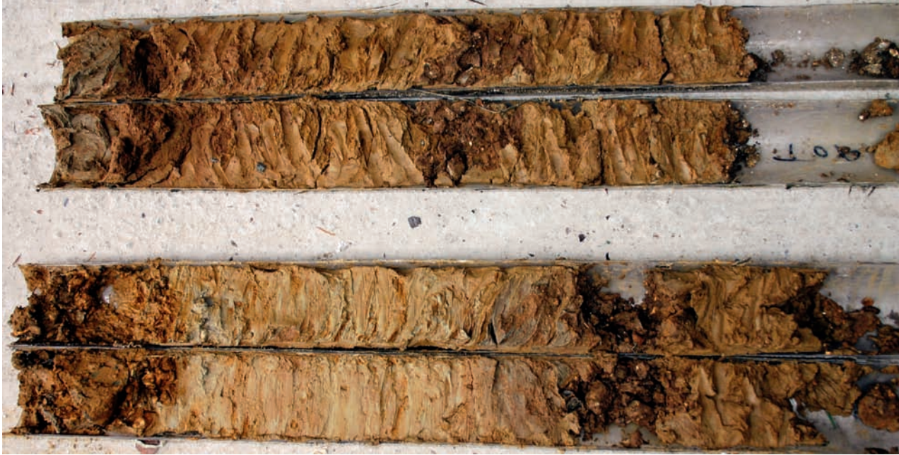
Fig. 2.5 Core samples from West Wittering. Cores are split to show stratigraphy. Fine grained sediments are estuarine deposits sandwiched between two cold stage gravels
