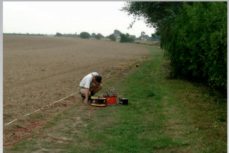
2.4.1 DC electrical survey equipment laid out along a transect at West Wittering, Sussex
