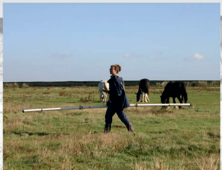
2.4.2 EM31 electromagnetic survey at Allhallows in the Medway Estuary, Kent
