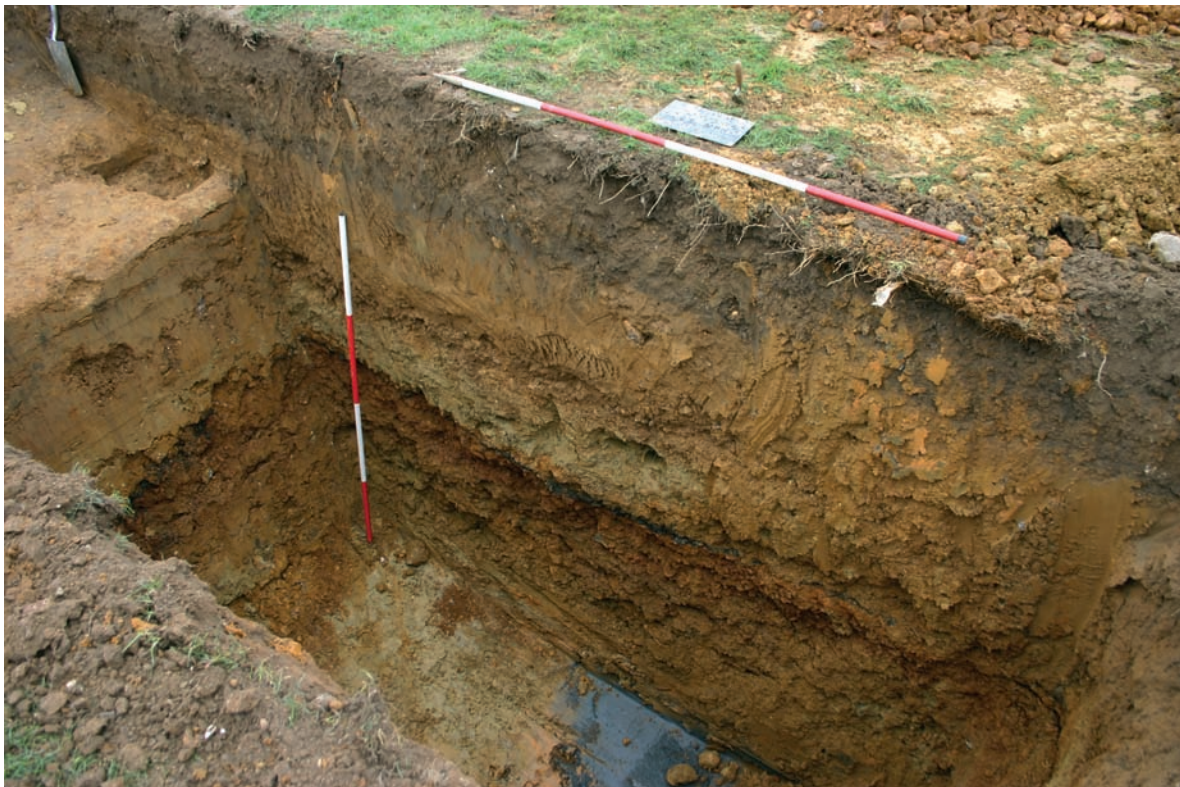
Fig. 2.12 Example of excavated test pit through gravels of the river Medina at Great Pan Farm, Isle of Wight
