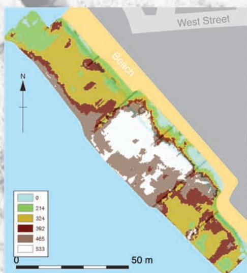
2.4.4 EM31 electromagnetic survey results from West Street, Selsey. Contour plot of conductivity values indicate a highly conductive zone equivalent with the position of the channel (Bates et al. 2009)
