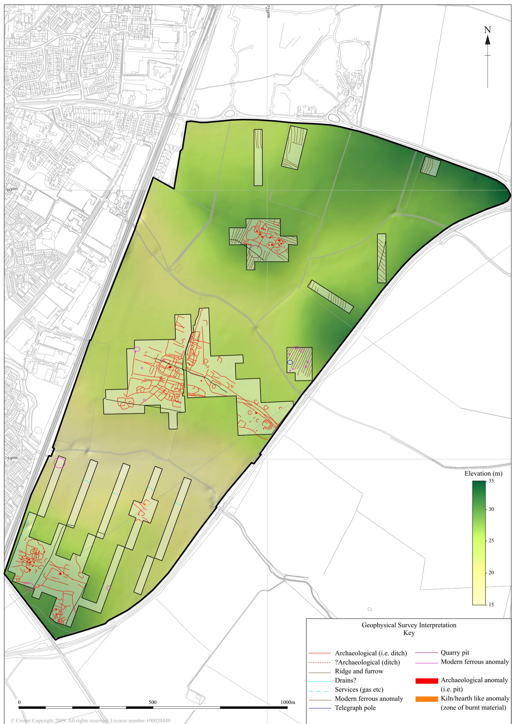
Figure 9: Topography and geophysical survey interpretations (scale 1:12,500)
