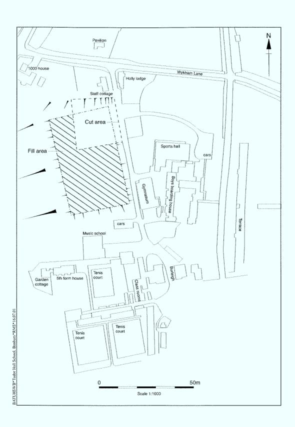
Figure 3: Plan showing probable cut and fill areas from construction of existing playing field.
