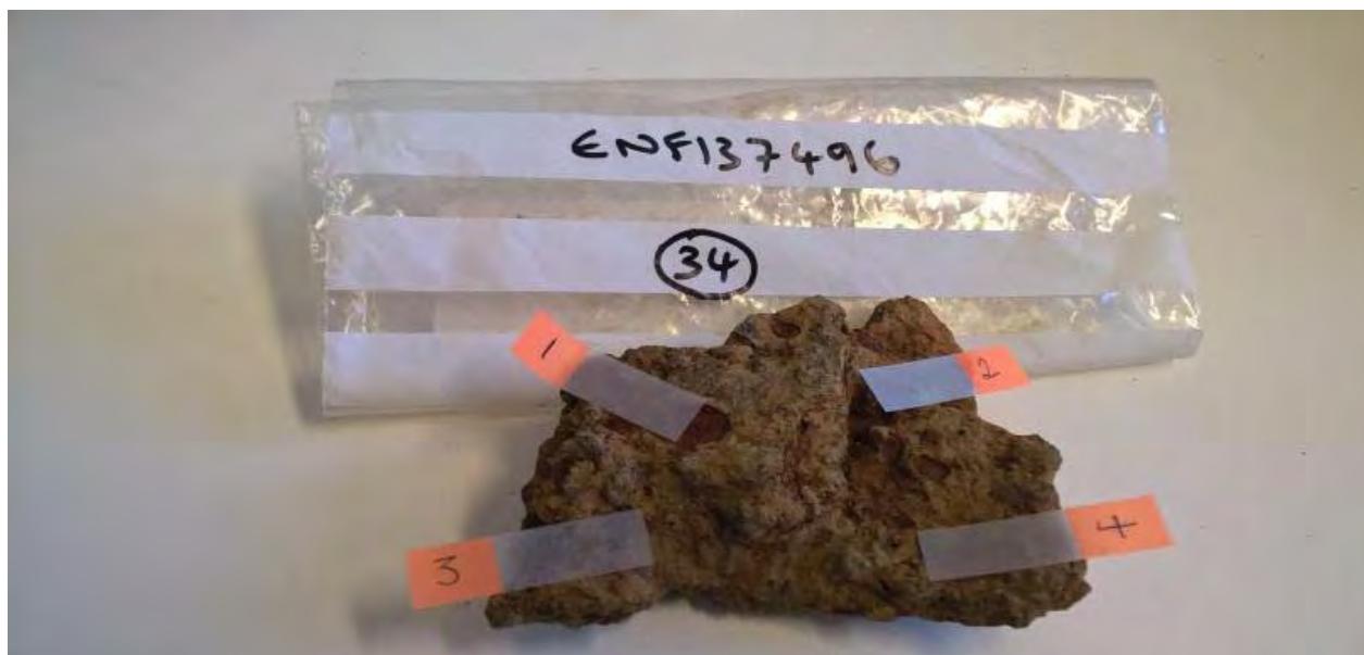
Appendix B.6 Plate 3: Salt slag from (34) – measurements 1-4
