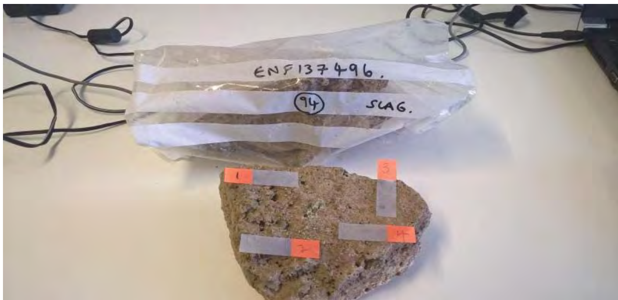
Appendix B.6 Plate 1: Salt slag cake from (94) – measurements 1-4
