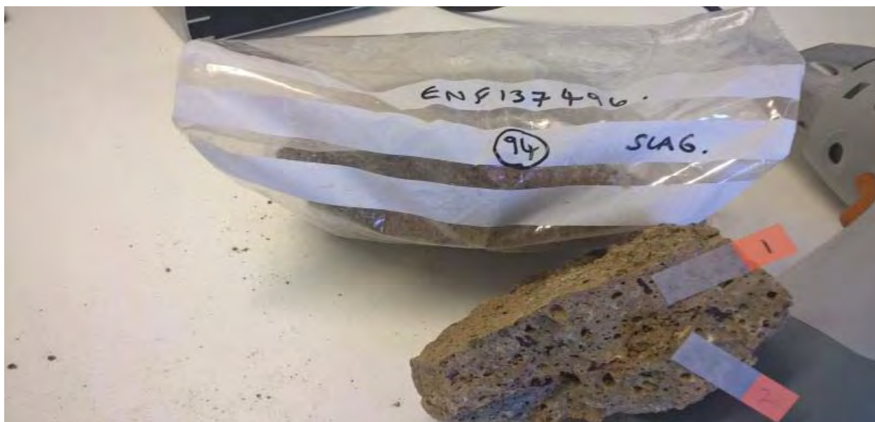
Appendix B.6 Plate 2: Salt slag cake from (94) – side measurements 1-2
