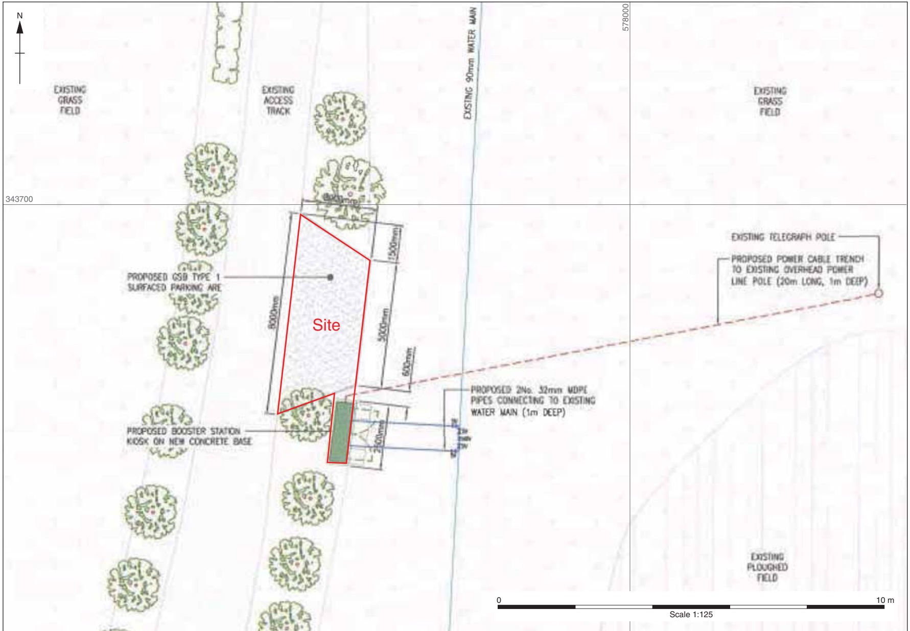
Figure 2: Proposed Booster station plan (Plan courtesy of Anglian Water)
