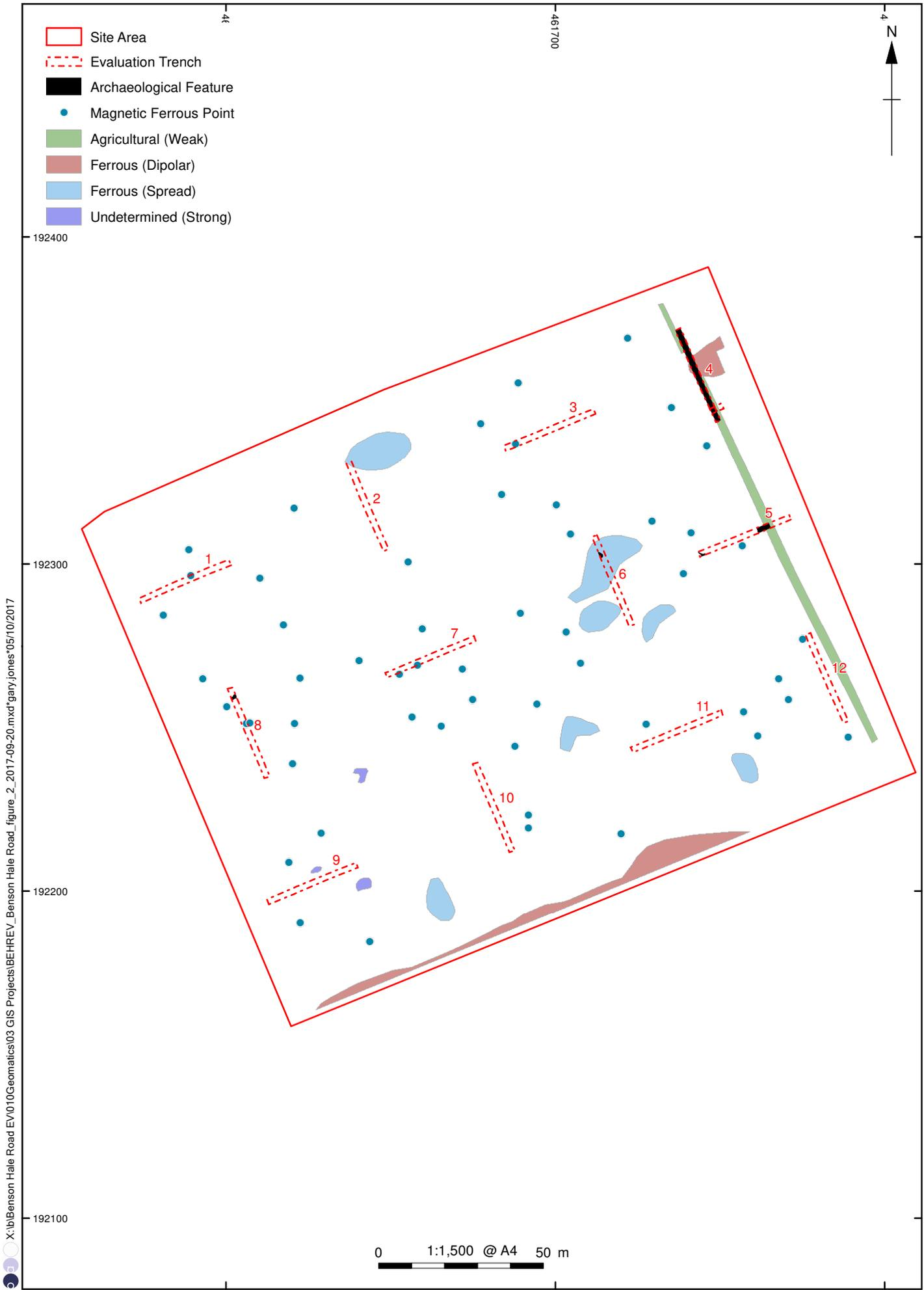
Figure 2: Trench layout with archaeological features and geophysical survey results
