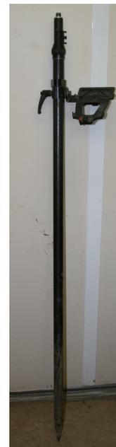
Slip the cradle on the pole, set the angle so you can look at the surface comfortably and tighten it up
