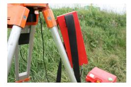
Clip the big red external battery to the tripod
