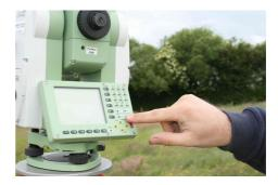
Press **shift** - **F12**. This will activate a laser plummet in the form of a red dot on the ground. Twist the feet on the tribrach to position the Total Station directly in the centre of the station point.
