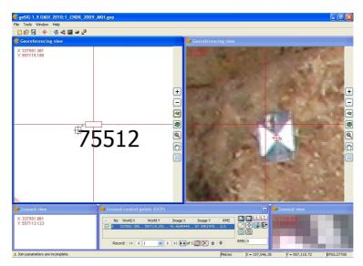
Use the "Previous zoom" or "-" tools above and below the "Zoom to select area" tool to select further points and repeat the above several times – at least three points are required, but a higher number increases the accuracy:
