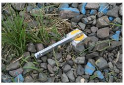
Spread the legs over the point so that the plate is level, and the hole of the screw over the point. Please note that the plate does not have an actual level, but that this is only for initial judgement by the eye.
