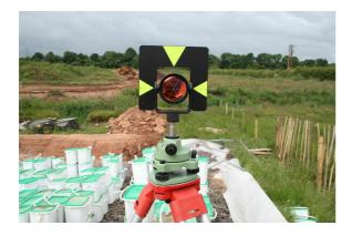
Look through the small viewfinder to the side of the tribrach and move it so the target is directly over the backsight point.
