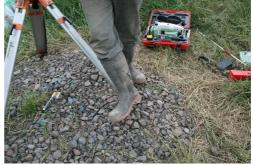
Undo the tripod legs and raise to roughly chest height. Tighten the screws / clips.
