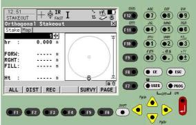
Hit "Shift", then "Conf" and ensure the option "Prefix" (this being "STKE") is selected – this differentiates the original points from the points staked out.
