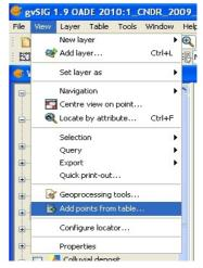
Now select the table you just added to the project from the drop-down menu. Define "Easting" and "Northing" as input locators and hit "OK" The points contained in the data-table will be displayed as a layer in gvSIG
