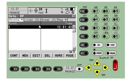
The STKE points will be surveyed without a code – use the data manager to change this manually. RP is the code that should be used.
