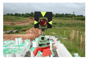
Open the orange box, and remove the circular prism. Turn the prism to face the Total Station on the station point.
