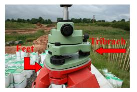
Do up the screw on the underside of the plate.
