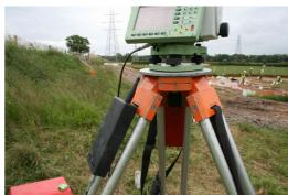
Press the 'prog' button to switch on the Total Station
