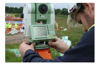
The front two feet are turned together, but in opposite directions, the back foot is turned by itself. Watch the screen as it will give you a numeric value to your machine tilt as well as having a useful picture to watch.
