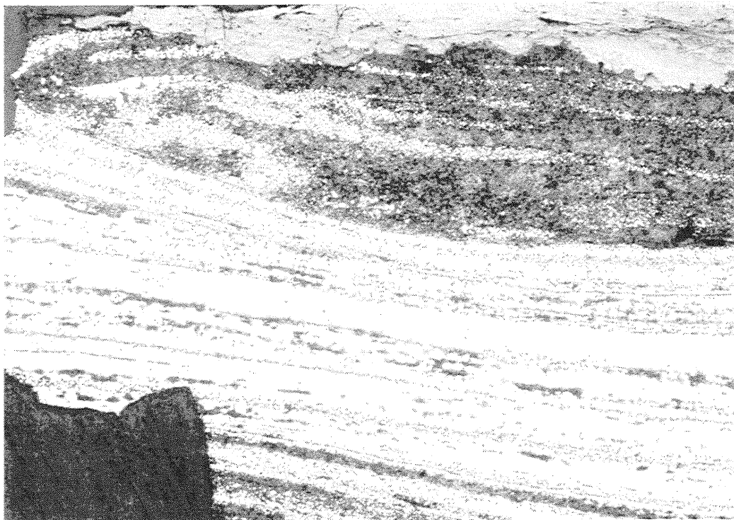
Fig 5: Photomicrograph of part of the banded structure in the section (HM 26A) from the back part of the single-edged knife. Magnification x 50; etched with 2% nital.
