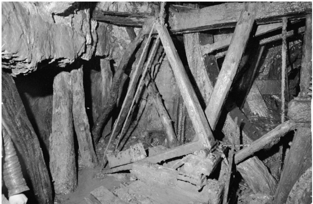
Plate 16: An example of a balance bob at the Ystrad Einion Mine (after RCAHMW ( www.coflein.gov.uk ))
