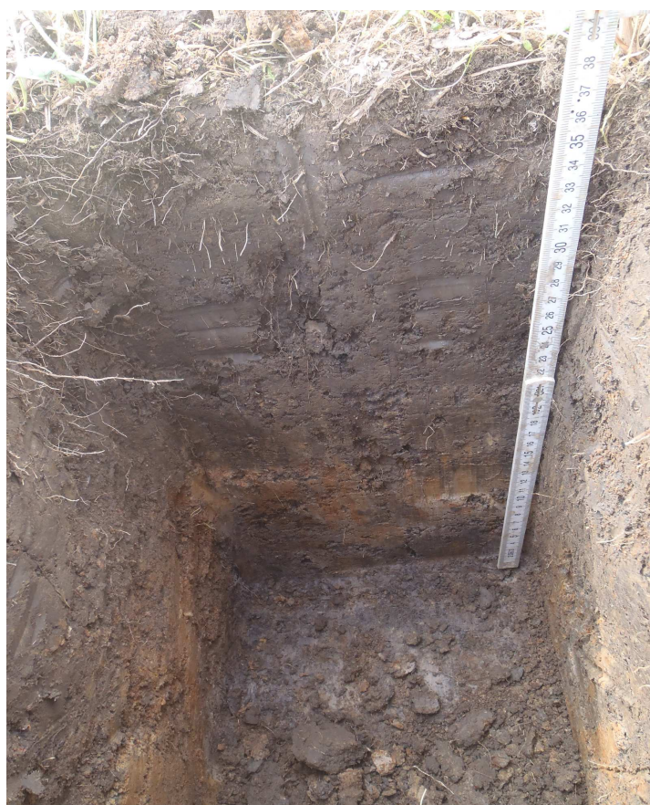
Plate 2: Representative stratigraphic sequence within test pit, showing topsoil over subsoil over the natural-occurring geology (clay)
