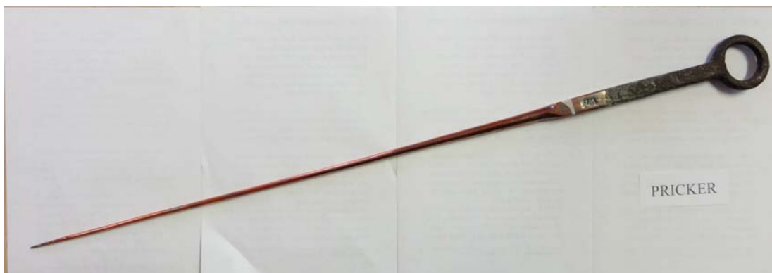
Plate 2: An example of a copper pricker used to prepare the fuse for a charge
