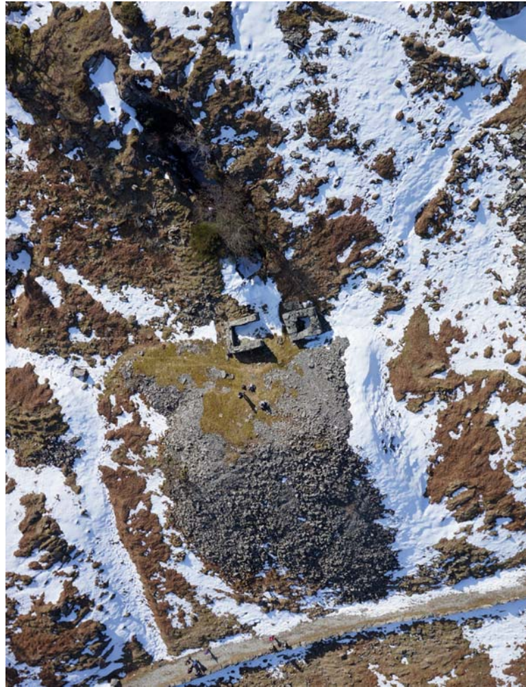
Plate 5: Aerial view of the Site 01 workings showing the quarry / adit, the riving sheds, the processing platform and spoil heap
