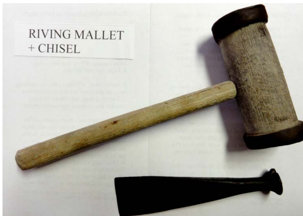
Plate 4: A riving mallet and chisel used to split the stone into thin slates
