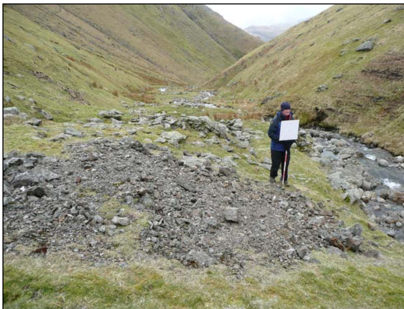
Plate 49: Detail of the spread of crushed ore on the main working floor 5
