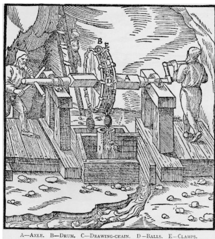
Plate 25: Example of a rag and chain pump drawing water through hollowed-out timbers (Agricola 1556)
