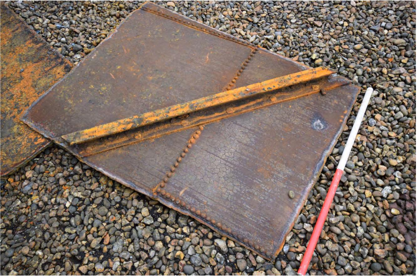
Plate 10: Ex-situ section of gasholder lift
