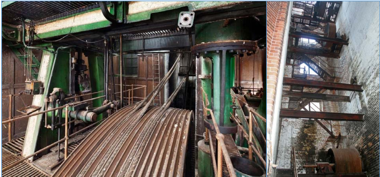
Plate 18: The fly wheel from a steam engine distributing power via a rope race (left) and an example of a rope race (right)
