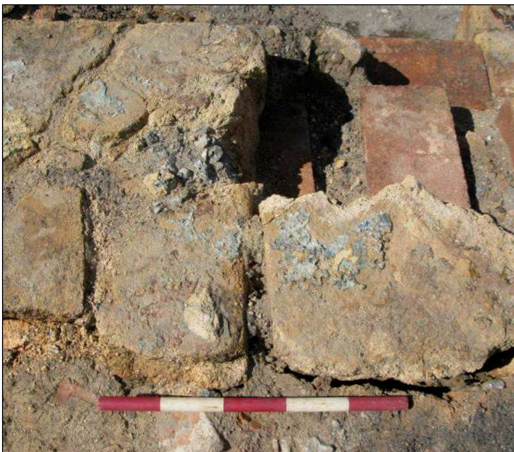
Plate 37: Vitreous deposits on the upper surface of refractory blocks 230
