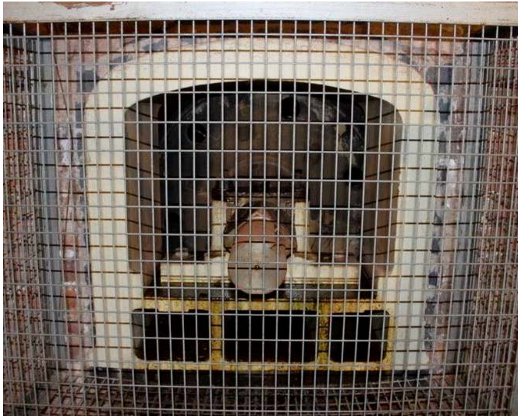
Plate 16: Large arched cast-iron bearing box
