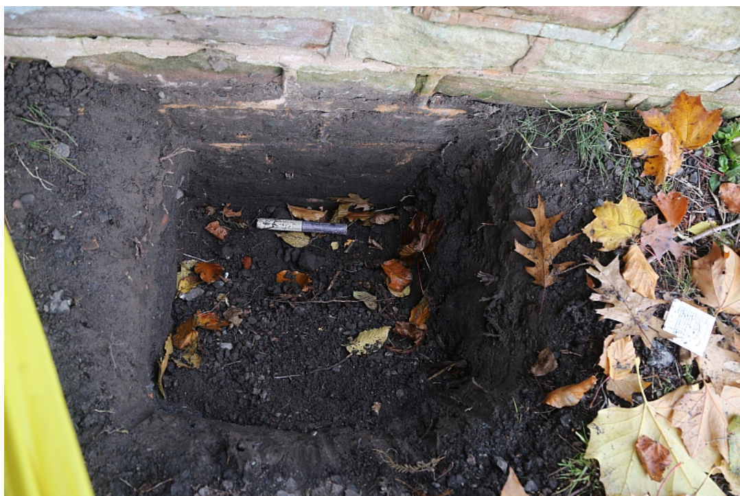
Plate 42: Representative illustration of test pits through the sandstone-built western part of the Ha-ha (TP2, 0.2m scale)
