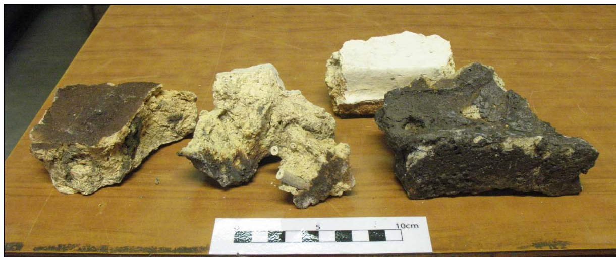
Plate 11: Fragments of the demolished muffle chamber, some of which show pipe-stem reinforcement. White clay washes are evident on the interior, as are steps in the wall thickness, forming peripheral shelves on which the bowls rested during firing
