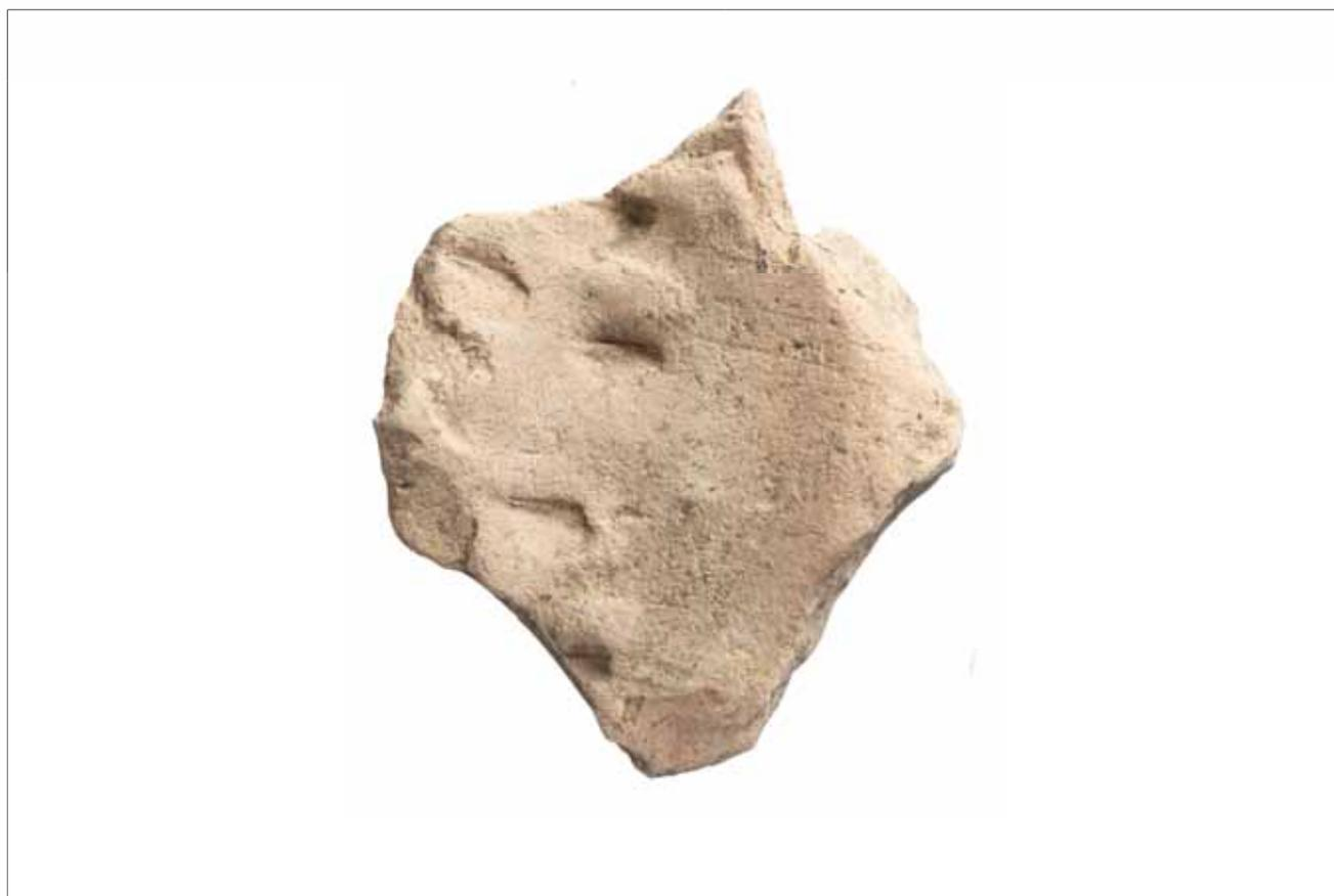
Plate B6.19: Internal surface of TGE saggur showing impressions of triangular props, pit fill 281, Phase 3, pit **279**
