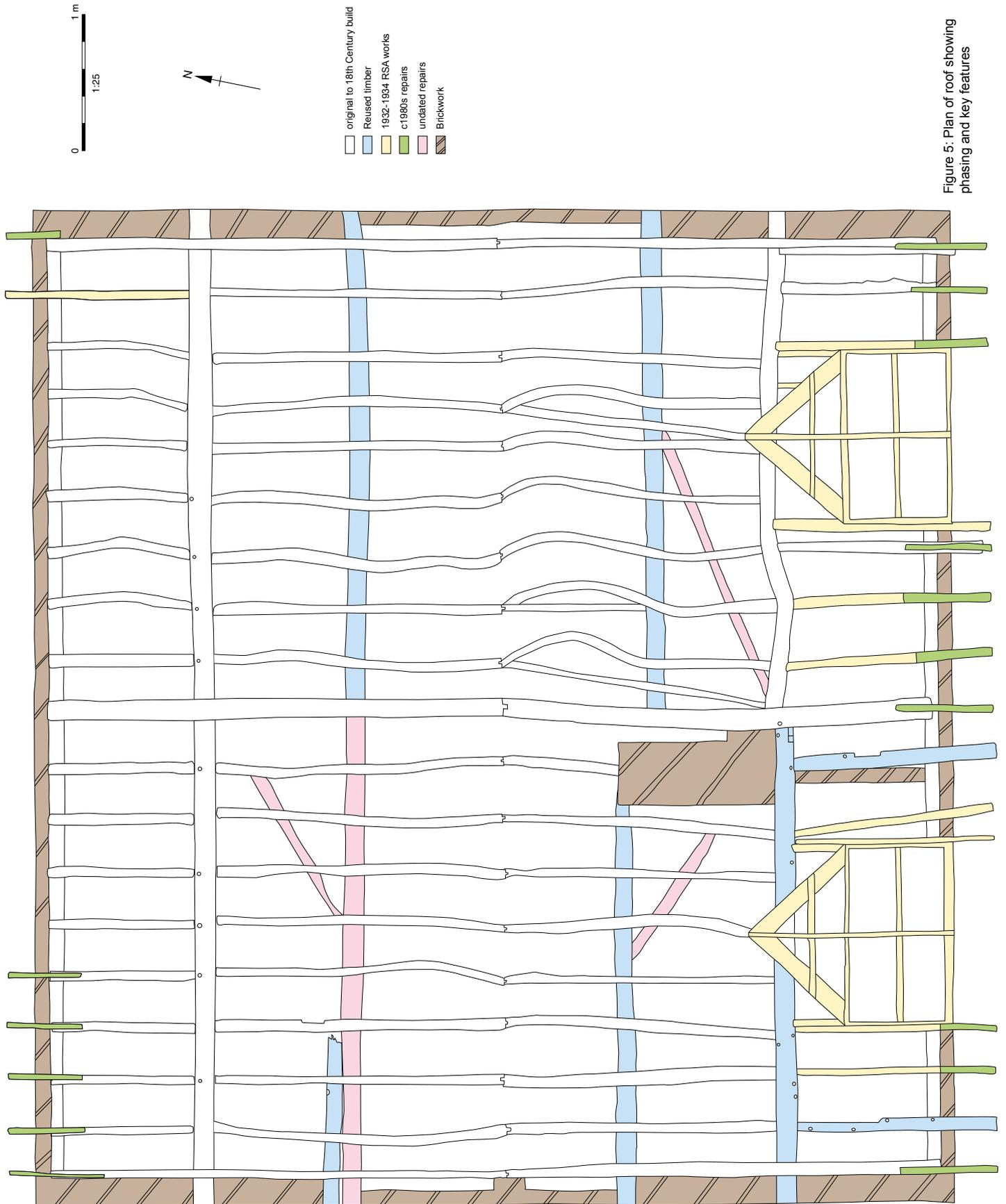
Figure 5: Plan of roof showing phasing and key features
