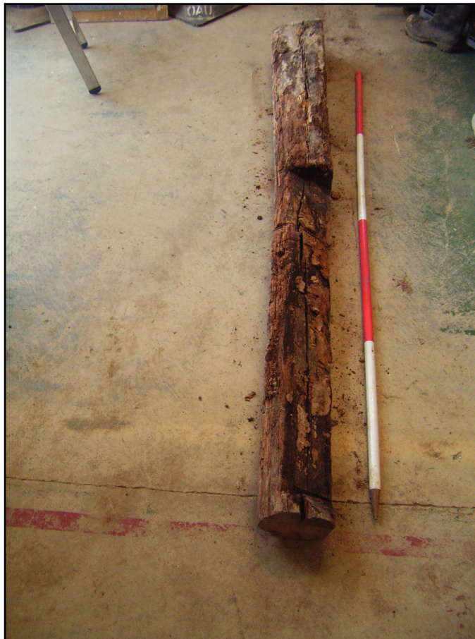
Plate 1: Timber removed from bastion showing angled rebate formerly above fireplace.
