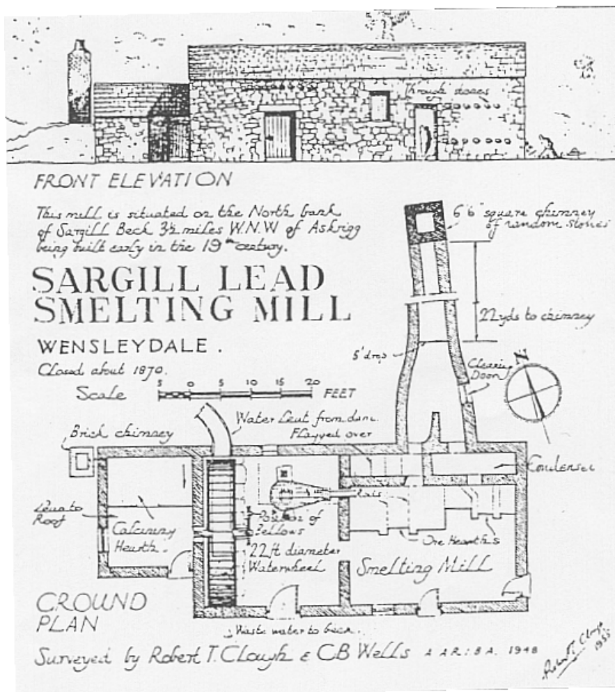
Fig 3 Smelt Mill Plan surveyed 1948 (after Clough 1962)
