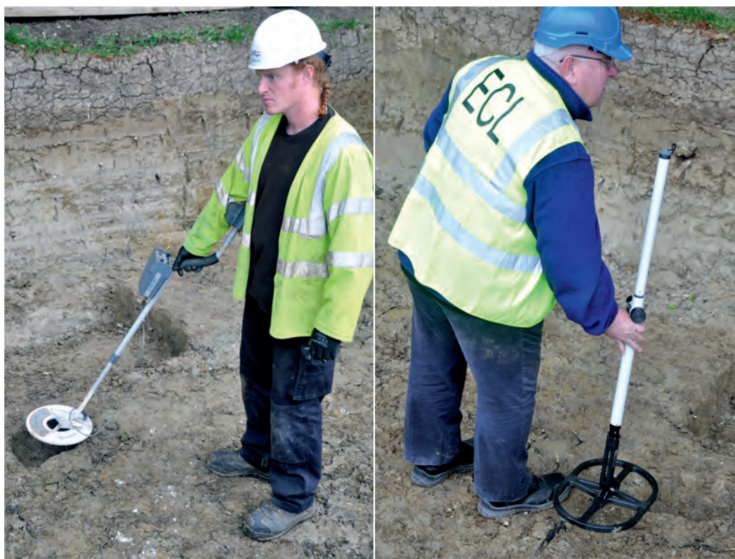
Fig. 2.13 Metal detecting for artefacts (left) and checking for unexploded ordnance (right)
