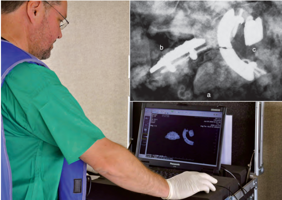
Fig. 2.25 Radiography of a soil sample showing how objects could be found. Inset: a) the eye of a hook, b) rising sun badge, c) 'Australia' shoulder title
